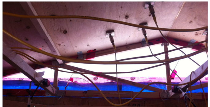
Strain gauge and pressure tap setup
