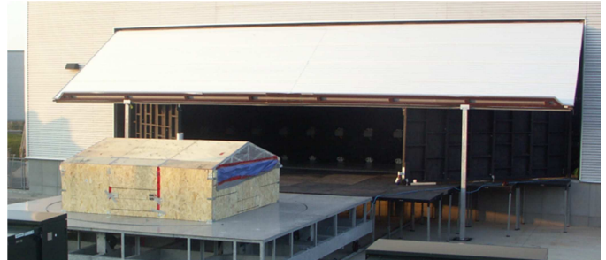
10' x 10' x 4' model being tested 4.5m away from the aperture of the contraction
